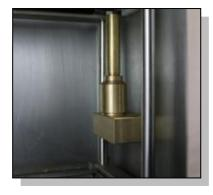
Inner Dia. Nozzle tube: 9.5mm
