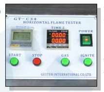
Counter 1: Igniting time Counter 2: flaming time Power switch Igniting switch Start/ Stop button Air source switch
